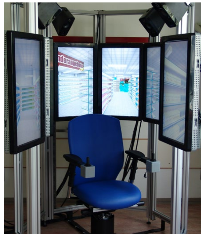
The training centre for the brain – a converted office chair and a ring of eight monitors create a 360° virtual supermarket.
