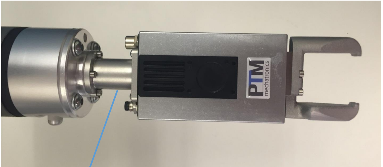
The active magnetic break is integrated in the robot flange
